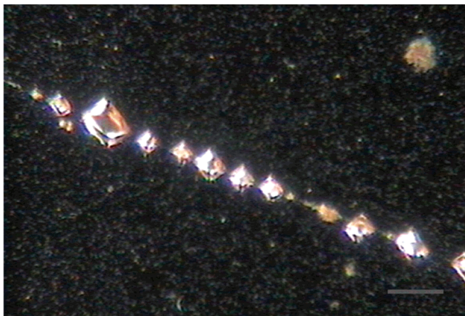
Figure 6. Optical micrograph (under crossed polars) of crystals formed on a diamond-like carbon film produced from poly(hydridocarbyne) on a silicon substrate. Processing conditions: thermolysis under argon to 1000 °C, ramp rate of 0.1 °C/min, held at 1000 °C for 24 h, and cooled to room temperature at 0.1 °C/min. Scale bar = 50 μm.
